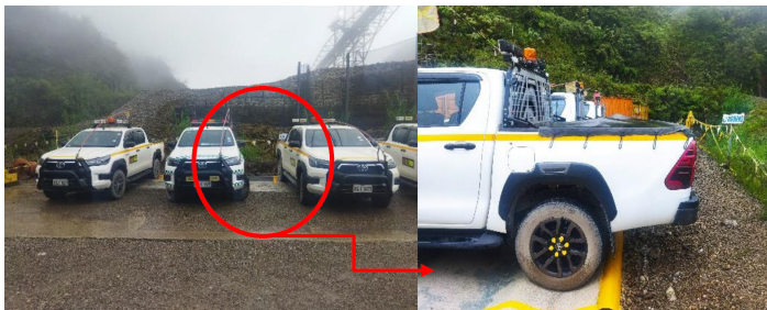
Figure 1. V-drains prevent uncontrolled movement
